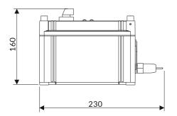
The box is made of polycarbonate. StandardEU62208,GOST. Impact resistance IK 08.
